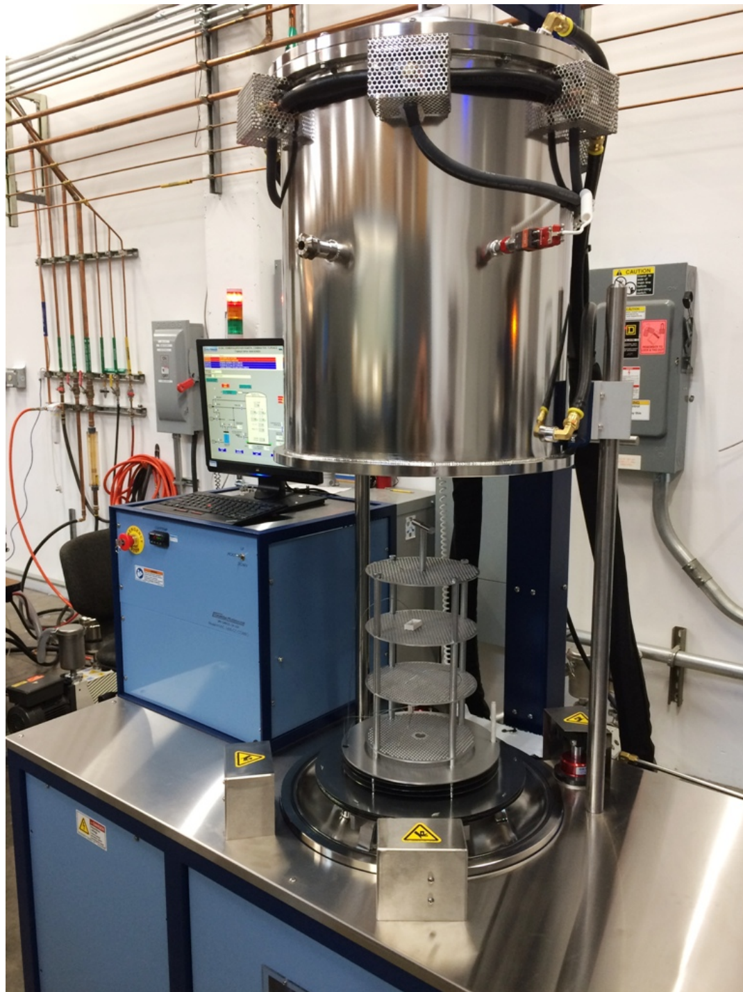
A Computer-Controlled Model H Furnace Shown open, with optional 4-shelf Molybdenum rack
